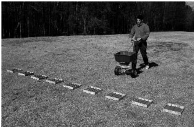
Figure 14. Pattern check for a rotary spreader.
