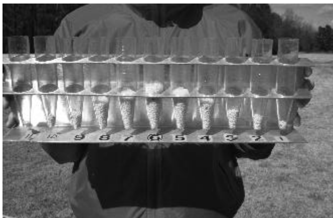
Figure 15. Rotary spreader distribution pattern in vials.
