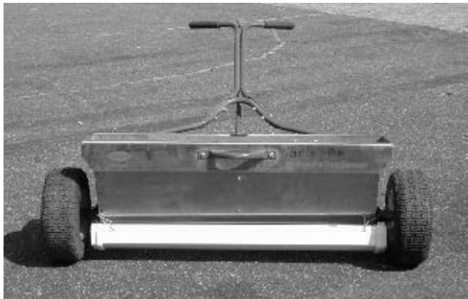
Figure 16. Drop spreader with catch pan.
