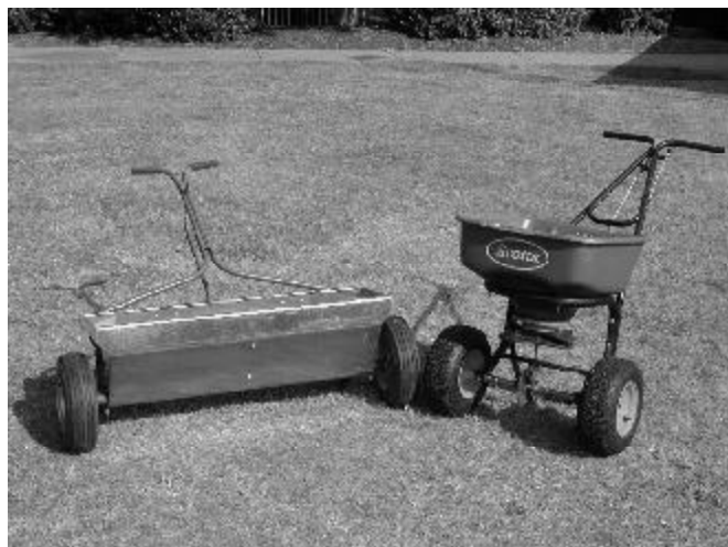
Figure 13. Drop spreader (left) and rotary spreader (right).
