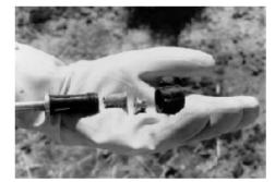
Figure 3.--Typical nozzle assembly.
