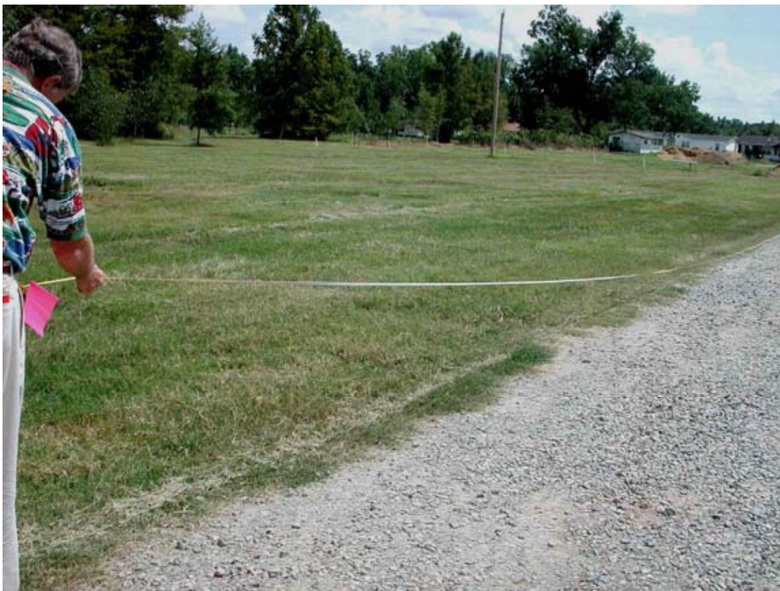
Laying out 100 ft distance for speed calibration.
