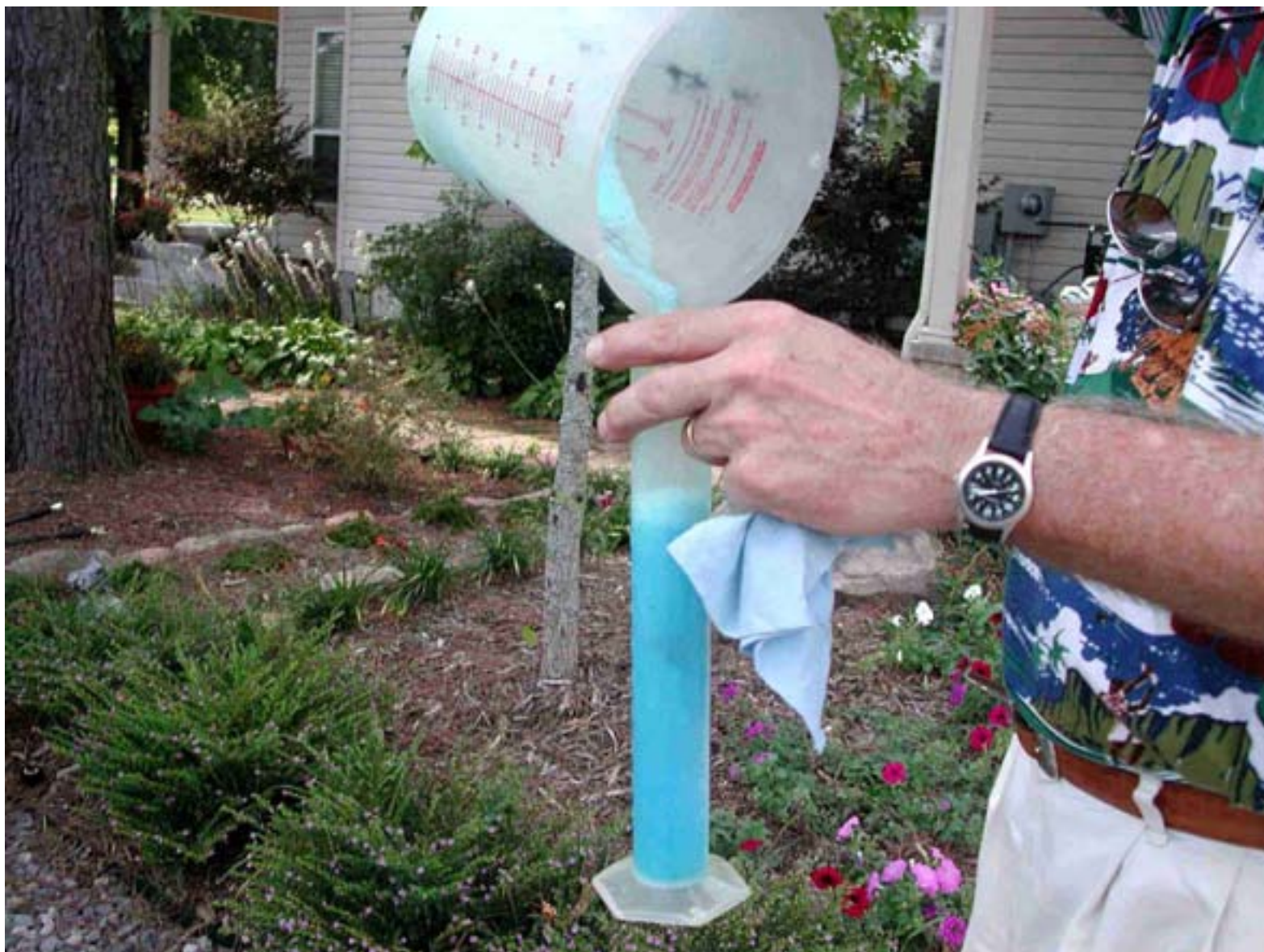
Measuring nozzle output with a graduated cylinder.
