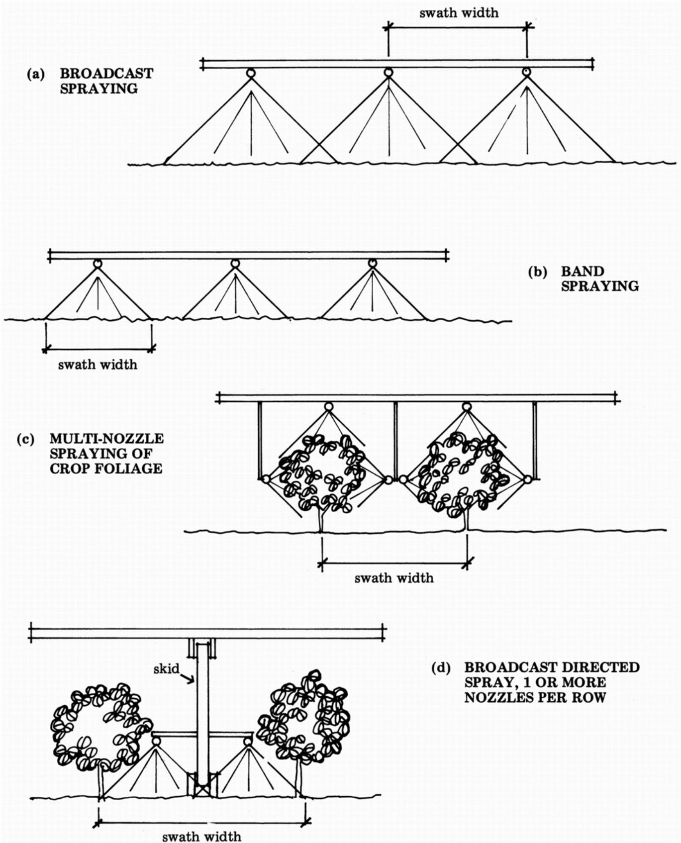
Figure 2. Swath widths for more common types of spray application.
