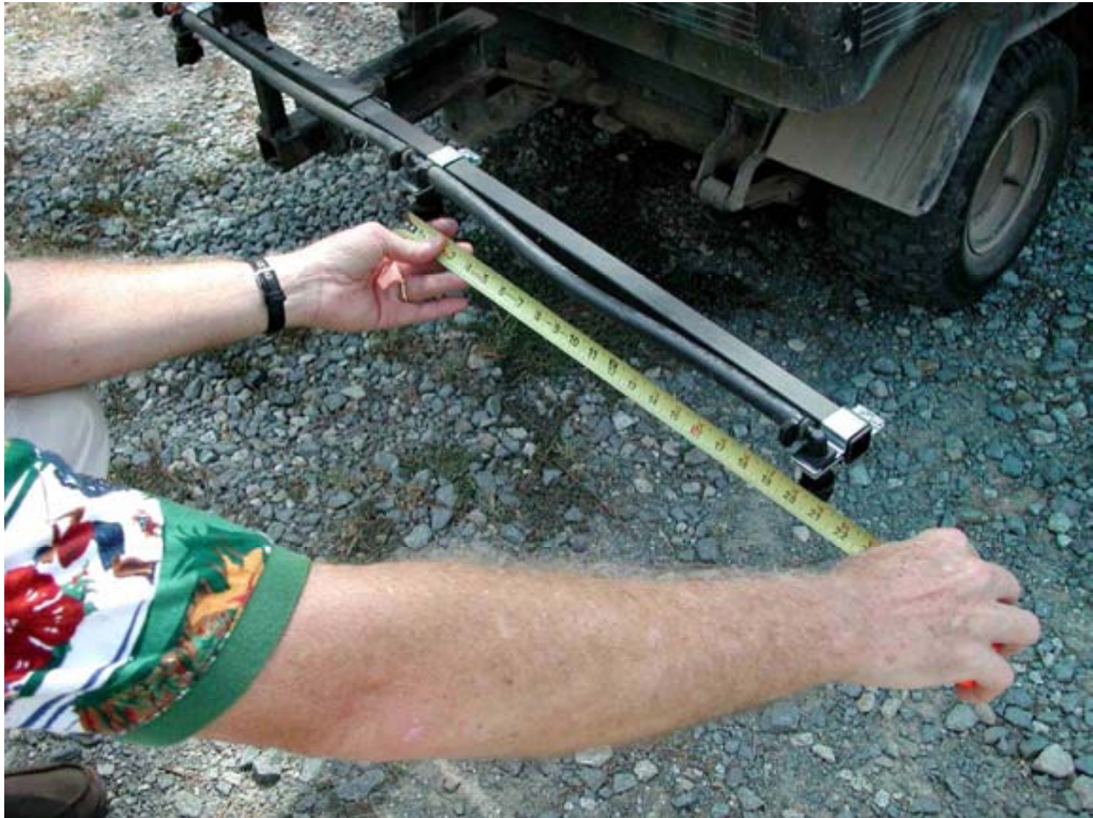
Determining nozzle spacing in inches.
