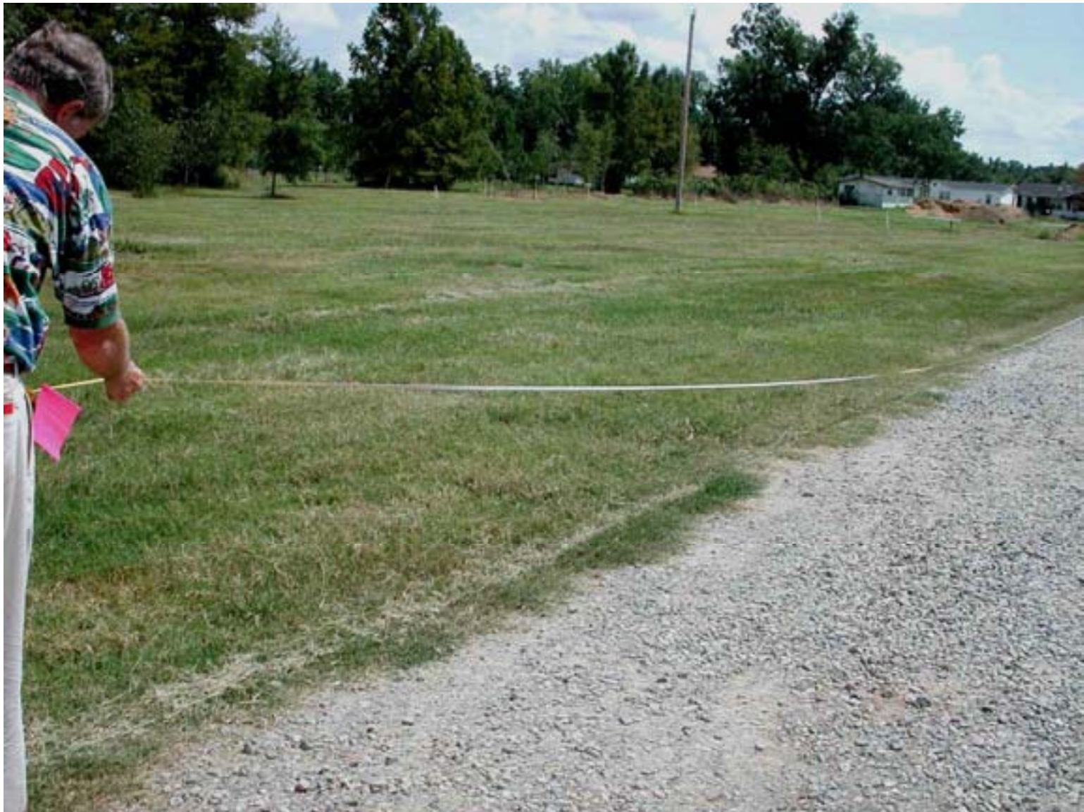
Laying out 100 ft distance for speed calibration.
