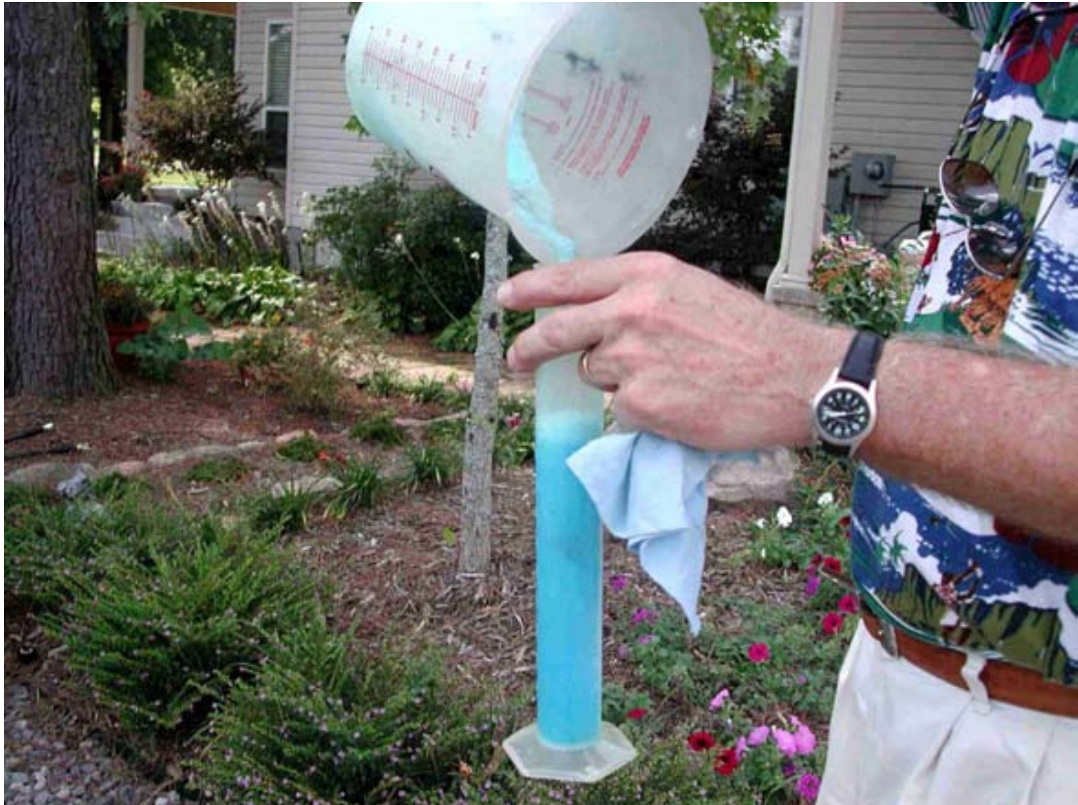
Measuring nozzle output with a graduated cylinder.
